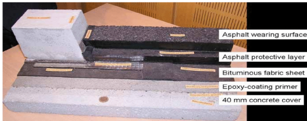
FIGURE 10 Bridge deck multiple-level protection system (16).
